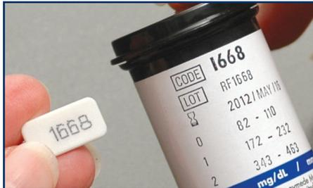
2. Insert Code Chip into your Meter with the numbers facing up.
